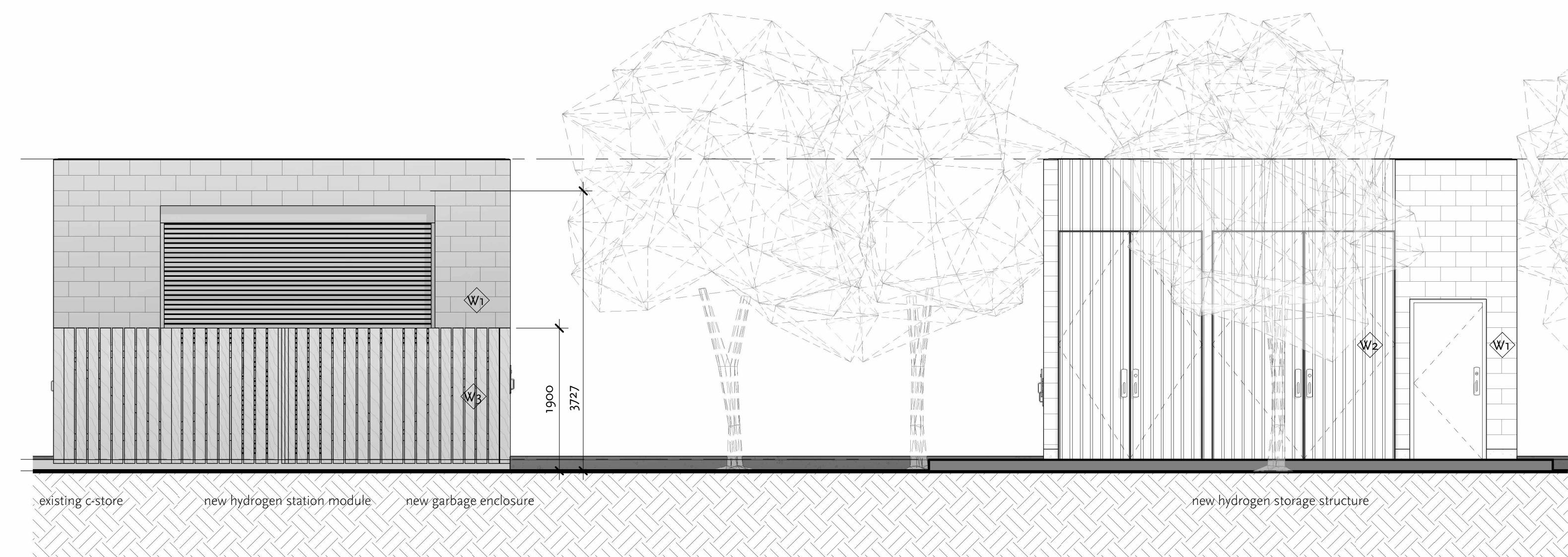
3 fenced yard and hydrogen storage structure - south elevations
