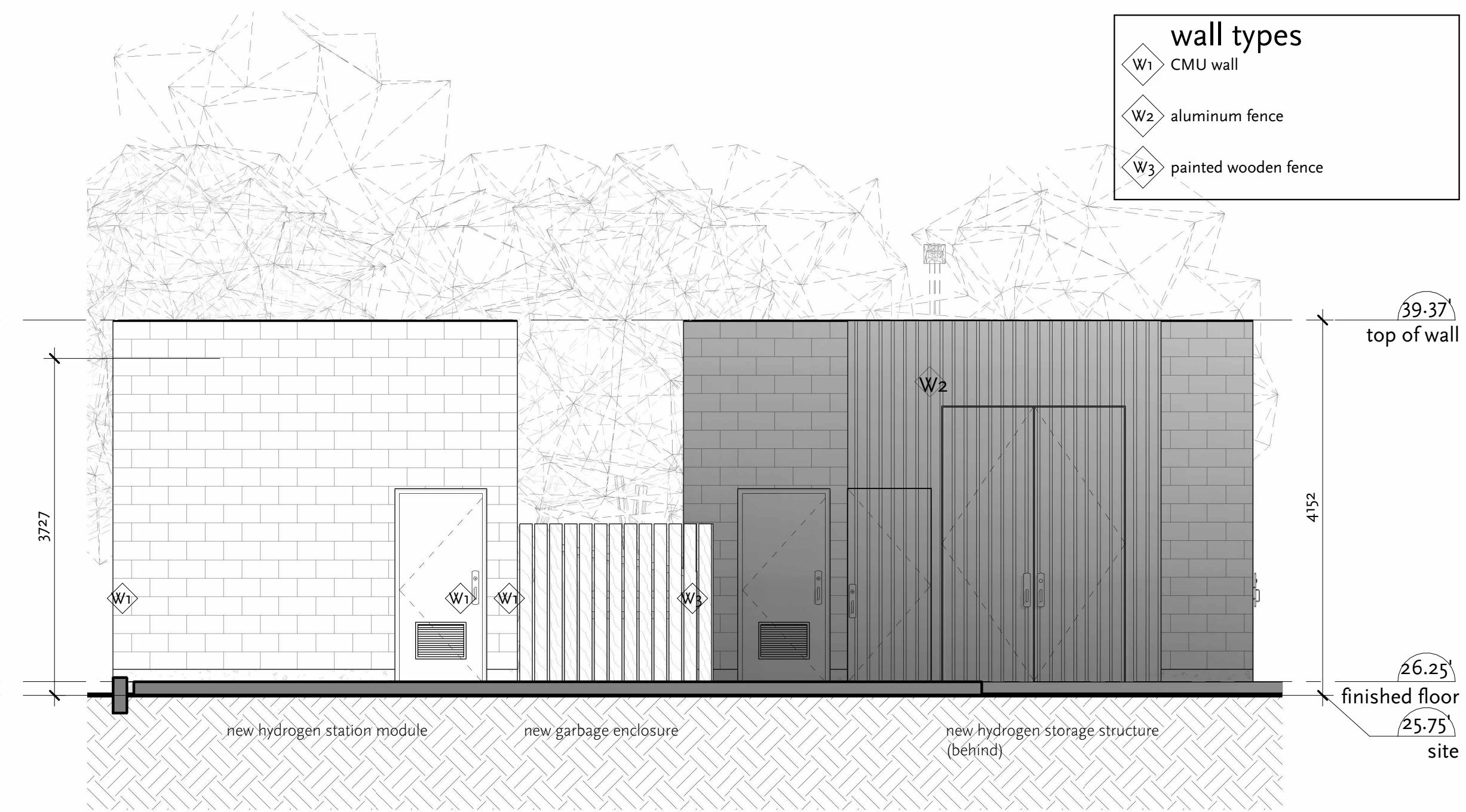
2 fenced yard and hydrogen storage structure - west elevations
